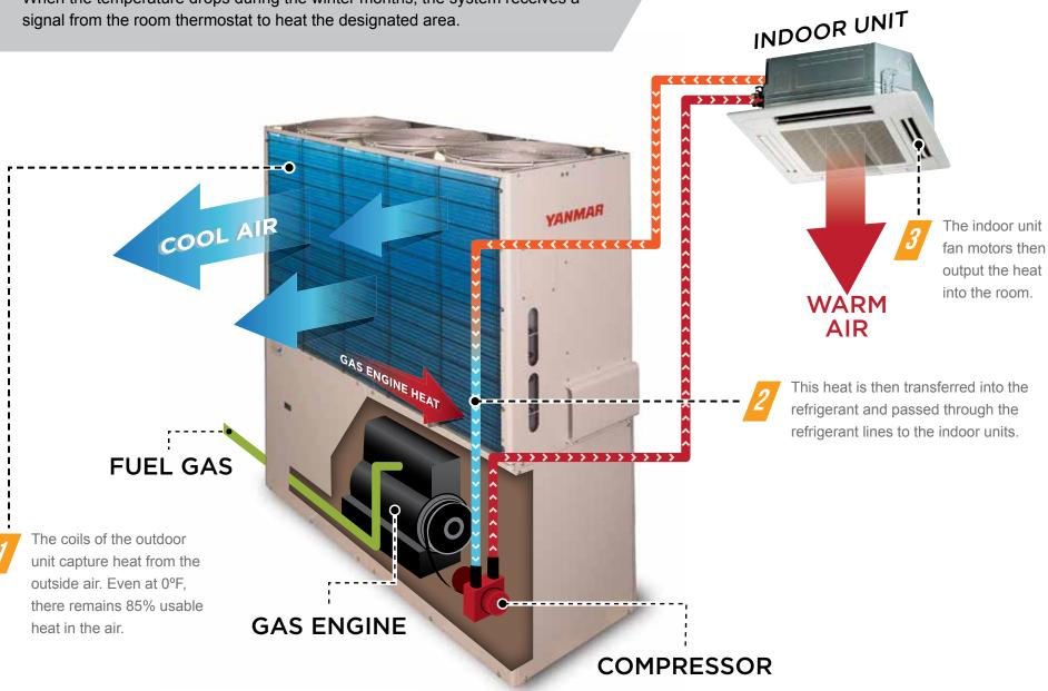
As temperatures reach or drop below 0°F, the heat created by the engine itself is also captured and cycled into the refrigerant circuit, effectively reducing energy consumption and costs.
